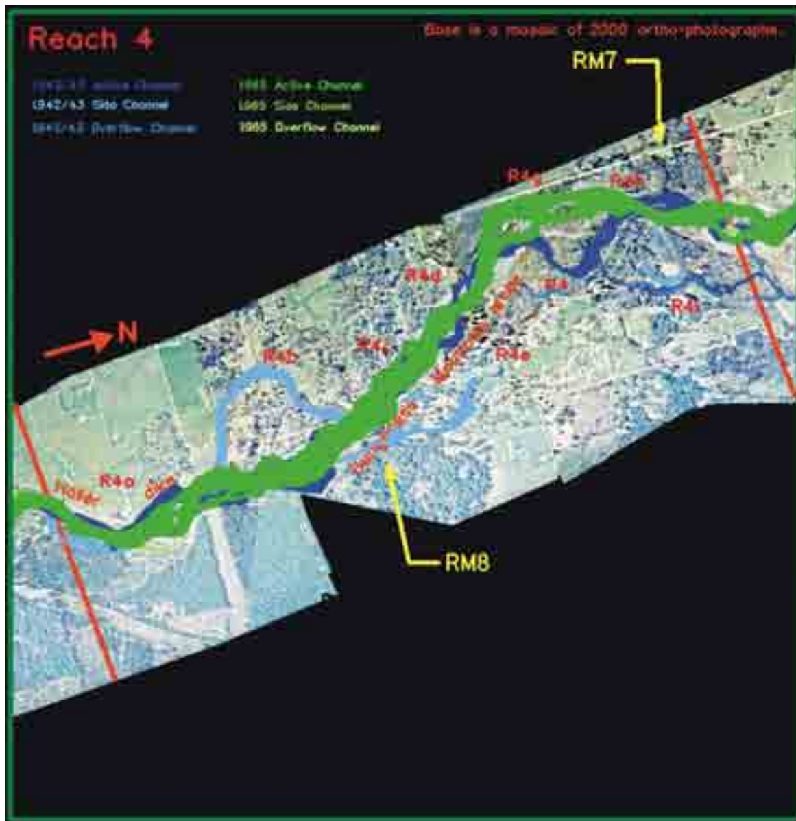
Figure O-7. Active channels, side channels, and overflow channels mapped from aerial photographs taken in 1942/43 and 1965 for Reach 4. Differences in the side and overflow channels may reflect their expression on the photographs rather than changes in the channels.
