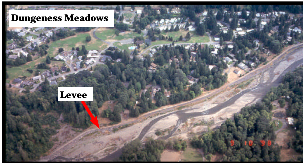
Photo 23: Levees have a large impact in the lower Dungeness River. The Dungeness Meadows levee (shown above) cuts off not only historic floodplain but also historic active channel (RM 7.5 to 8.5). The levees also increase flow depth, velocity, slope, and sediment transport capacity. This also results in the removal of large woody debris that could otherwise form stable log jams and scour pools. Bars are elevated in this reach due to the higher river stage caused by the levee. The Dungeness Meadows levee was extended downstream to block the entrance to a side channel and prevent flooding in the subdivision. To increase fish utilization while still protecting homes from flooding, the lower portion of the levee could be setback to the east side of Spring Creek. Another option would be to create a small opening in the levee that would limit flows but allow fish passage. Photo taken 9-10-98.
