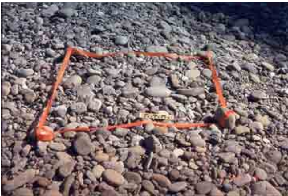
Figure D.2. Surface of unvegetated gravel bar at Sample Locality DRsed-5B downstream from Woodcock Bridge. Our 1-meter square sample area was delineated by the flagging tape on the bar surface. The pavement was composed chiefly of gravel and cobbles and was about one particle diameter thick at this location. This pavement was excavated, sieved, and weighed before the underlying bed material was sampled.
