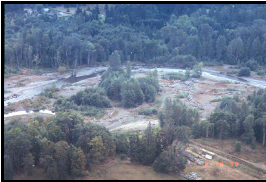
Photo 10: As the river migrates, sediment from the bank is eroded and added to the total sediment load. The majority of bank materials are formed of river sediment deposits (sand and gravel) with a layer of silt on the surface. Photo taken 9-10-98.
