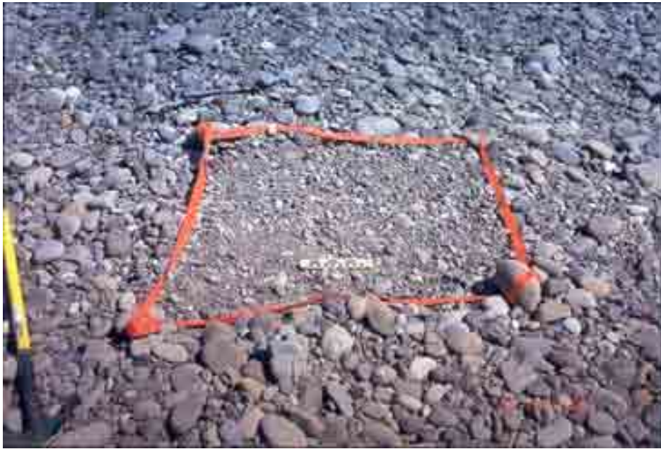
Figure D.6. Example of bed material exposed following excavation of the surface pavement layer at Sample Locality DRsed-5B. The thickness of the pavement was about one particle diameter at this location. The bed material beneath the pavement was markedly smaller than the pavement and is more representative of the material carried in the bed load of Dungeness River.
