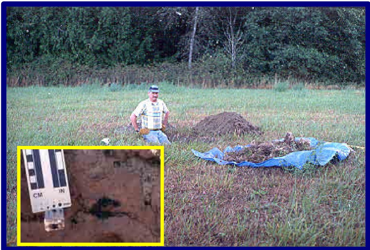
Photo 13: Natural exposures were excavated and used describe soil development. Where present, charcoal was collected and analyzed by radiocarbon dating. These dates along with soil development and geologic mapping helped identify the ages of terraces along the Dungeness River and establish the natural boundaries of the active river channel over the last several thousand years. Photo taken 9-13-98.
