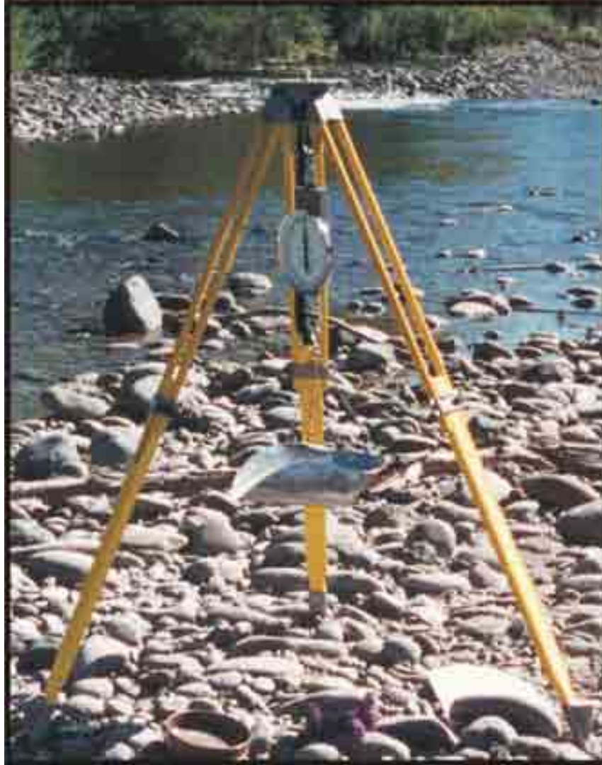
Figure D.5. View showing the scale suspended from a tripod which was used to weigh the sample in each size fraction. Samples too large for the pan were weighed in smaller portions and a cumulative weight was then calculated for the entire size fraction.
