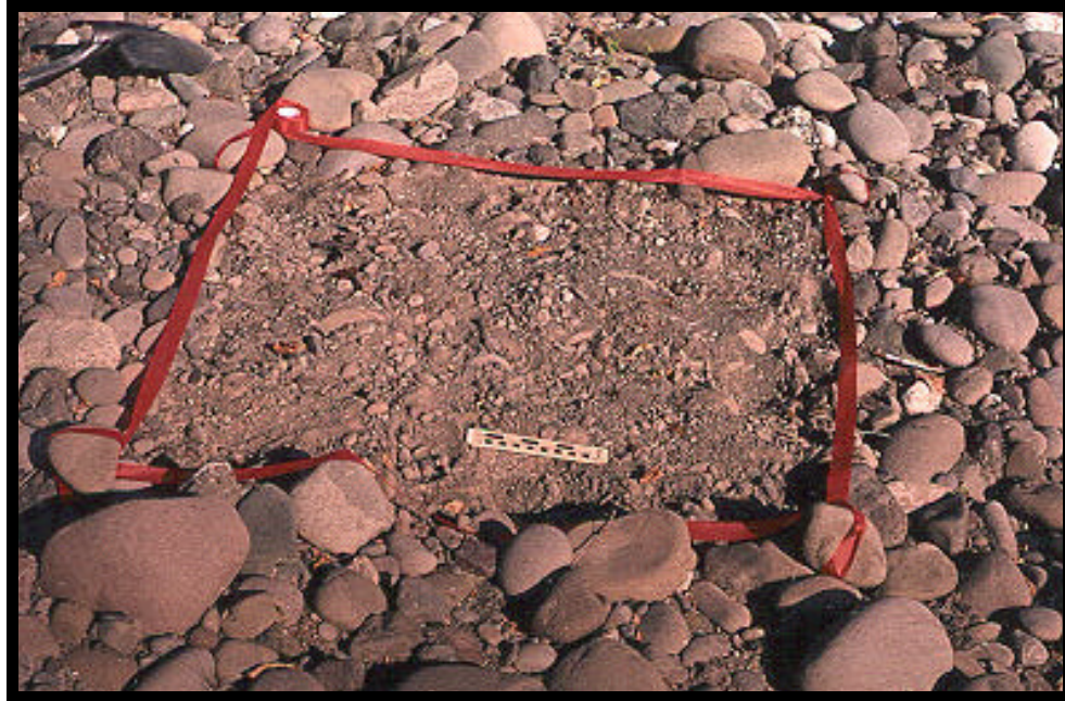
Photo 11: Bed-material samples in gravel bars were taken in 3-ft (1-m) squares to determine the sizes of sediment present in the river channel. Analysis of the samples showed that the channel bed of the Dungeness River is typically composed of sand, gravel, and cobble-sized material. The sand-sized particles are typically present beneath a pavement layer of cobbles. In general, the size of the bed-material decreases in the downstream direction. Photo taken 9-9-98.
