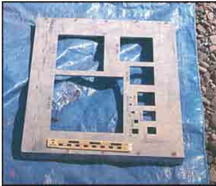
Figure D.3. Gravelometer, or pre-cut template, used to sort particles larger than the 32-mm sieve. The smallest opening through which a particle passes determines its size group. Size groups measured with the gravelometer were 32 to 63 mm, 63 to 90 mm, 90 to 128 mm, 128 to 180 mm, and larger than 180 mm. Rocks larger than 180 mm were weighed individually and then totaled to obtain the weight for that fraction.
