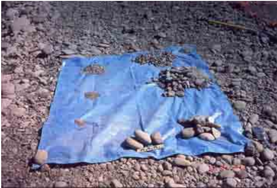
Figure D.4. Sediment from pavement material at Sample Locality DRsed-5B separated into the following size fractions (counterclockwise from bottom center): 90 to 128 mm, 63 to 90 mm, 32 to 63 mm, 16 to 32 mm, 8 to 16 mm, 2 to 8 mm, and finer than 2 mm. After the sediment was separated into fractions, each sample was weighed in order to determine the distribution of particle sizes within the pavement.
