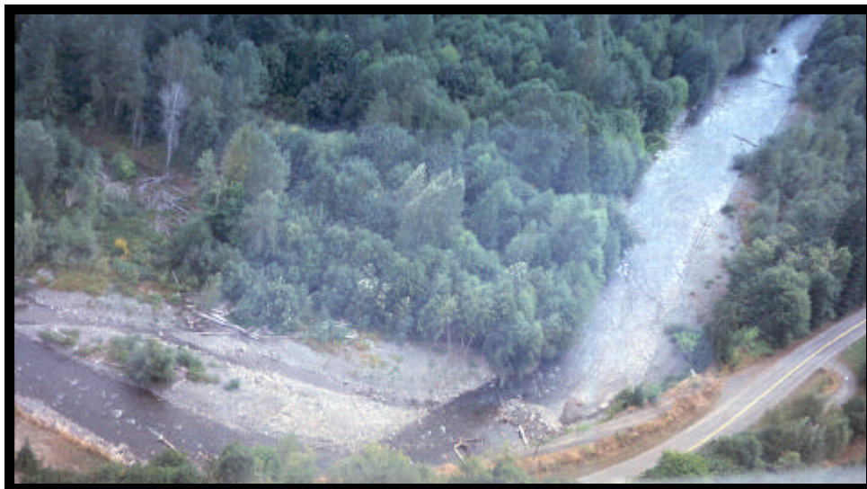
Photo 21: On the west side of Kinkade Island, the main channel has migrated to and eroded a portion of a high glacial deposit. This erosion forced Clallam County to setback the road. Further erosion was prevented by the placement of large angular boulders at the base of the slope. Photo taken 9-10-98.
