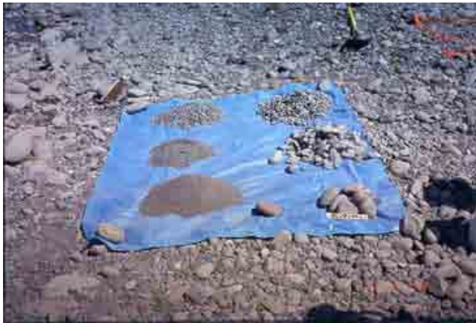
Figure D.7. Sediment from the bed material at Sample Locality DRsed-5B after separation into size fractions. Each fraction was individually weighed to determine the distribution of sizes within the sample. Compare the size fractions in this photo with those shown for the overlying pavement in Figure D.4.
