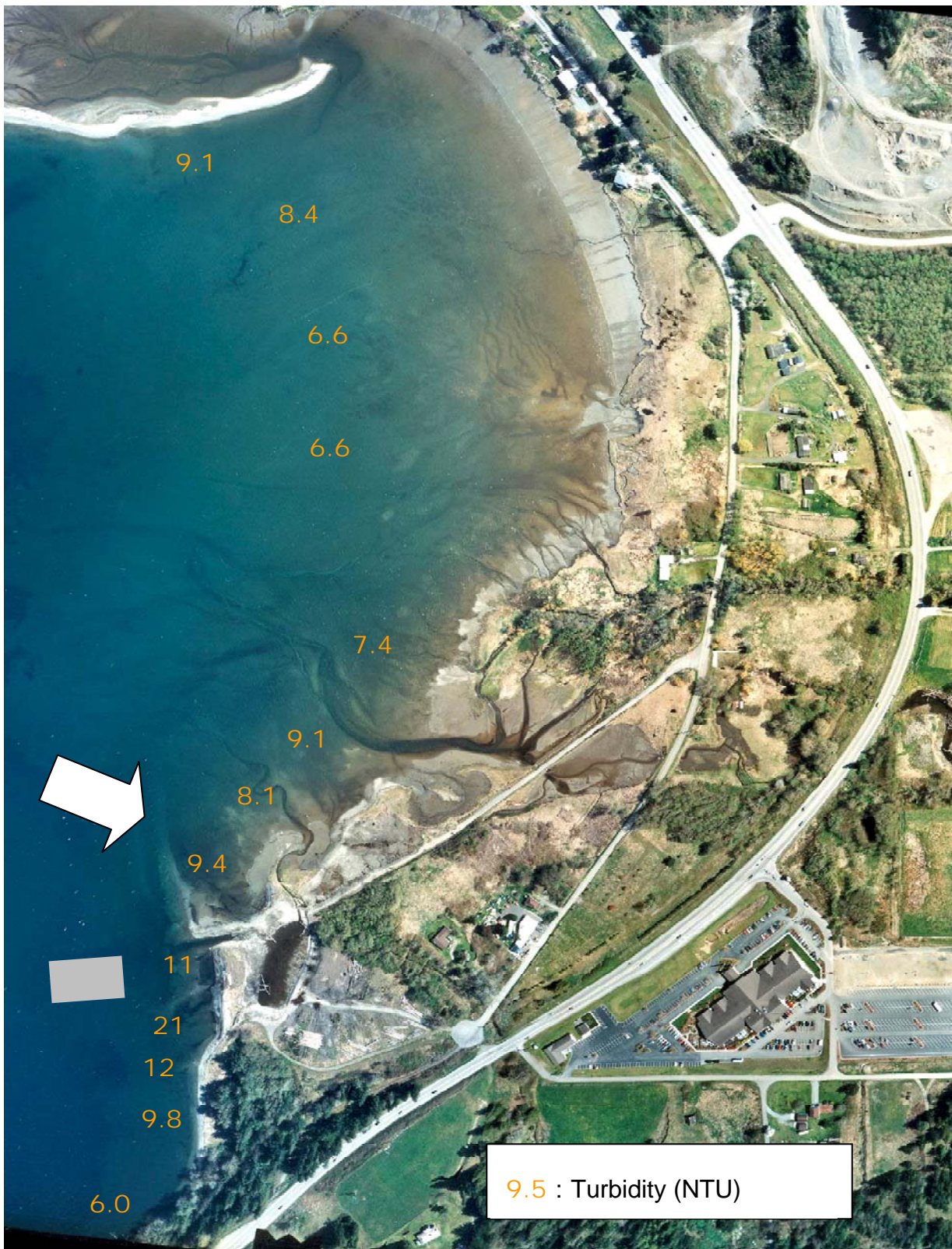
Figure 4.9. Turbidity reading recorded along a transect across the south end of Sequim Bay after approximately 8 hours of piling removal activity. Orange values indicate turbidity (NTU). White arrow indicates direction of water movement. Grey rectangle represents position of barge at the time of the transect.
