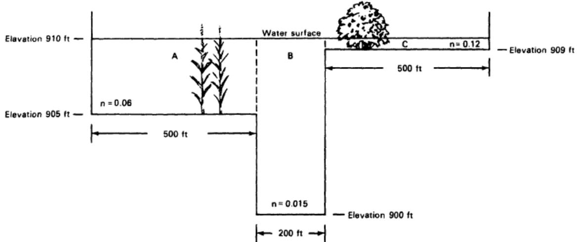
**Figure 1.6. Sub-section discharge method diagram. An example of how peak discharge was calculated. (Jobson and Froehlich, 1996). The Cowan method ( $n = (n_0 + n_1 + n_2 + n_3 + n_4)m_s$ ) was used to determine the roughness coefficient “n” of each sub-section (Cowan 1956).**
