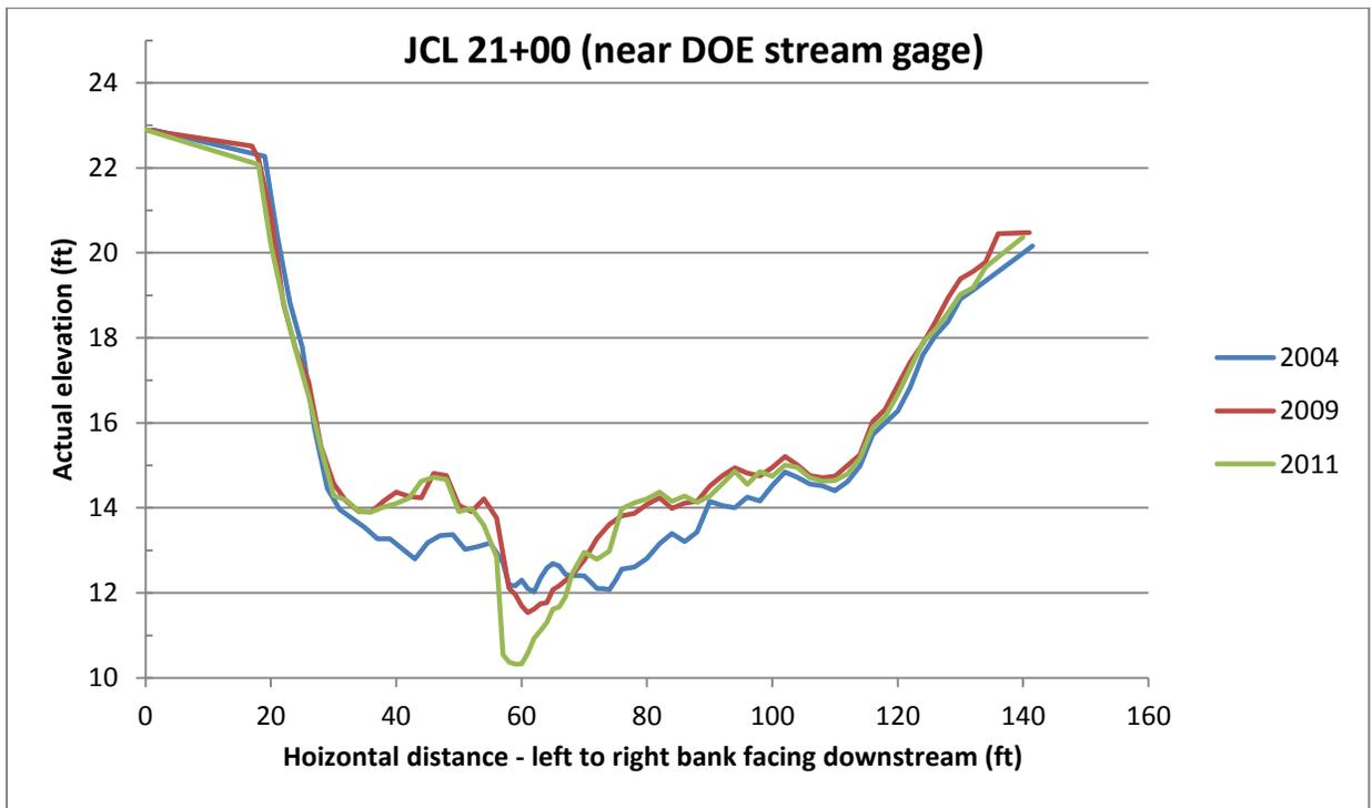
Figure 2.8. Sample JCL channel cross-section (JCL 21+00) for the years 2004, 2009 and 2011.
