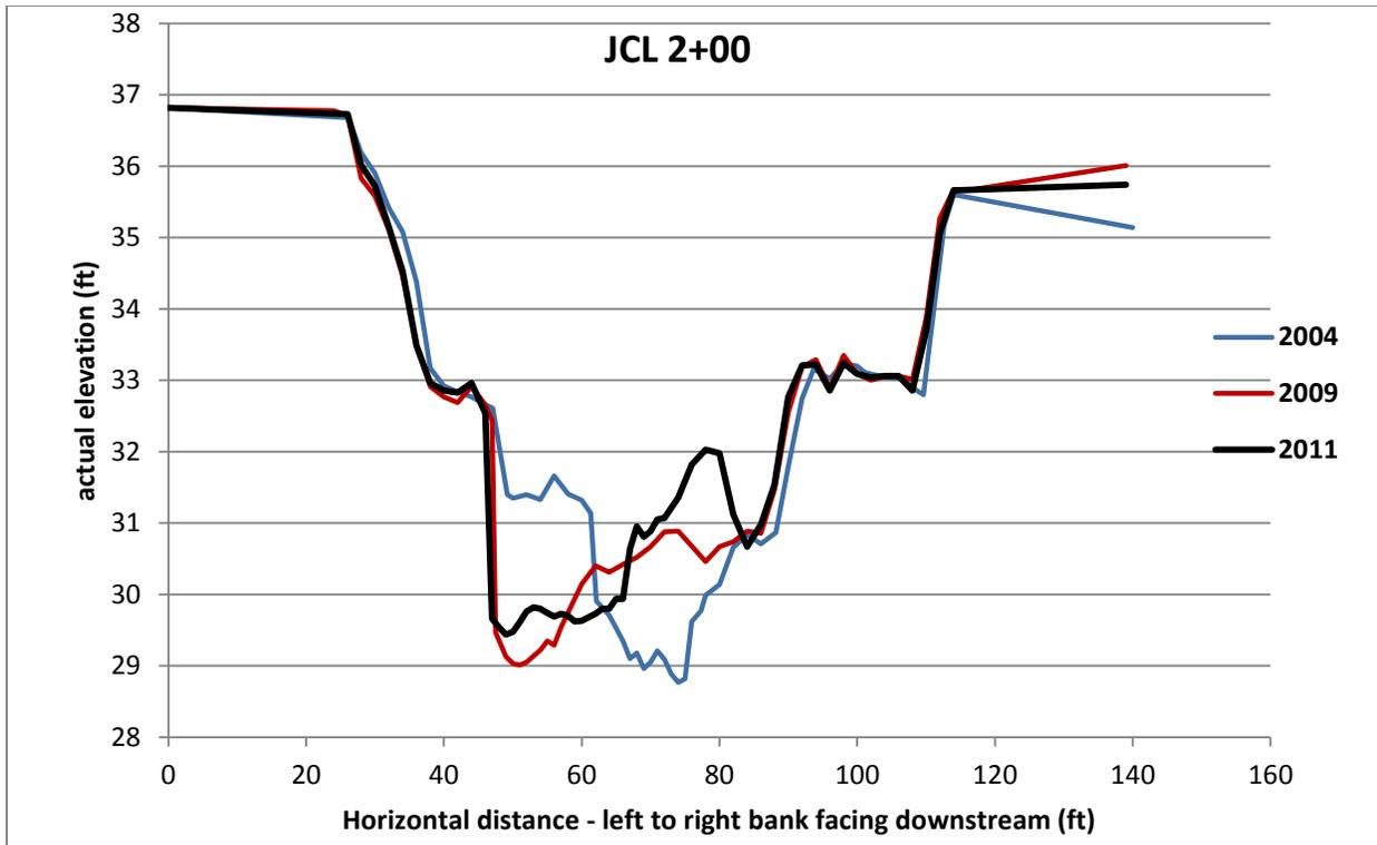
Figure 2.5. Sample JCL channel cross-section (JCL 2+00) for the years 2004, 2009 and 2011.
