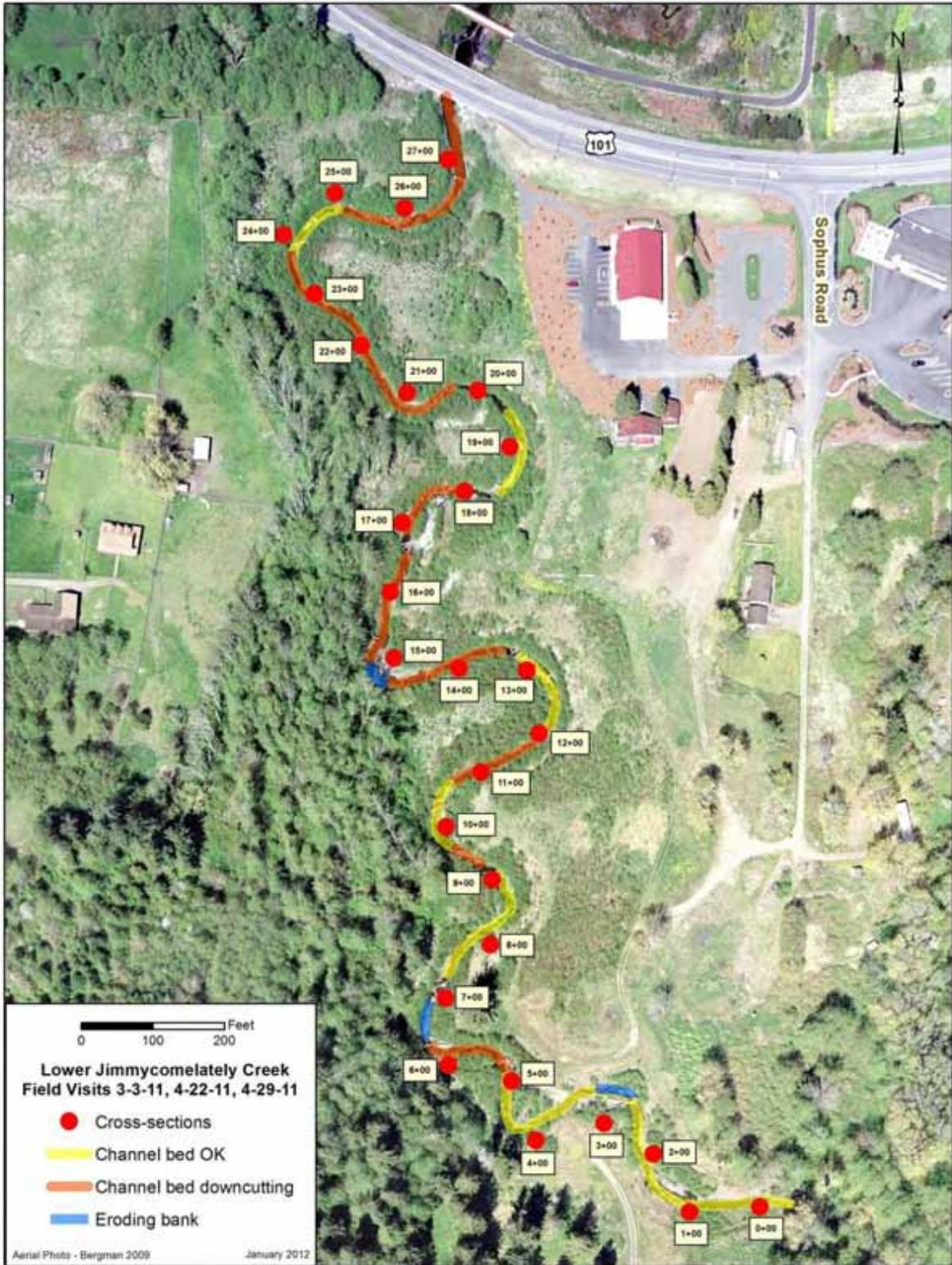
Figure 2.4. Areas of the JCL Creek channel where the channel bed is stable (yellow), downcutting (orange), and eroding (blue), based on March and April 2011 field visits (Graphic by Pam Edens).
