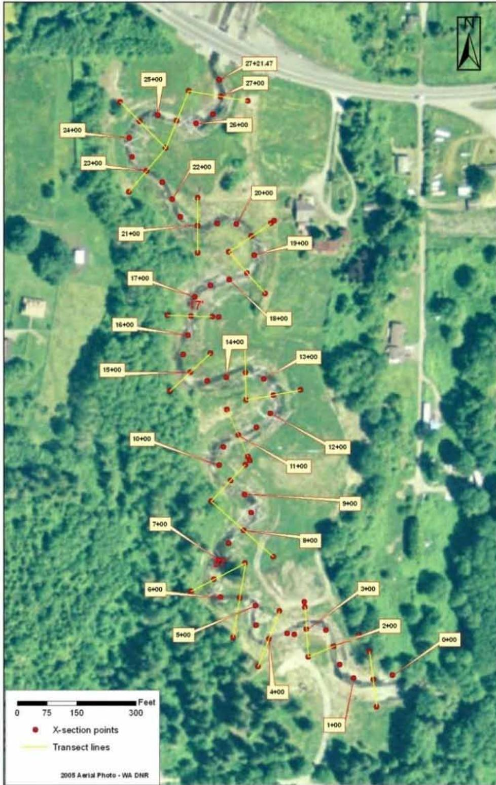
Figure 2.1. Location of JCL Creek channel cross-sections. To interpret the numbering, 2+00 is 200 ft. downstream of the upstream end of the channel realignment project (Graphic by Pam Edens)
