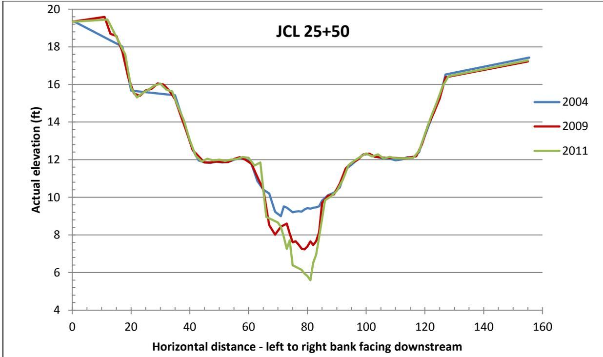
Figure 2.9. Sample JCL channel cross-section (JCL 25 + 50) for the years 2004, 2009 and 2011.
