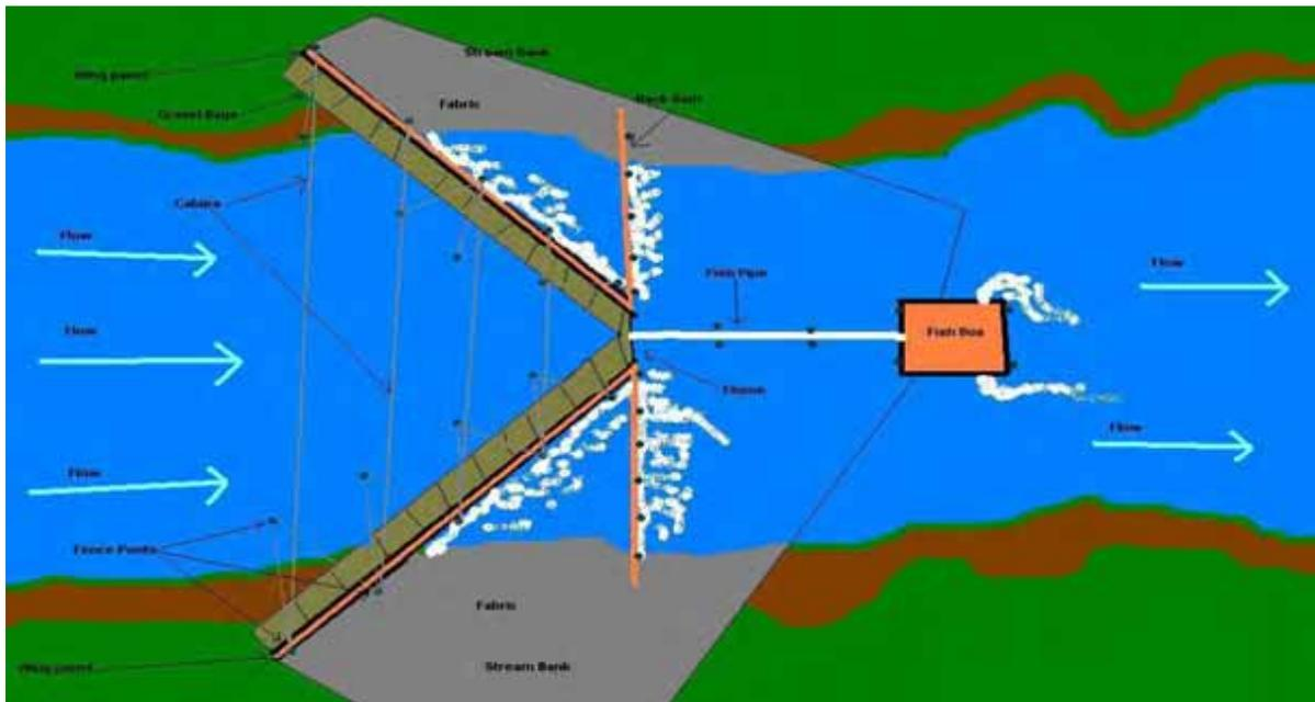
Figure 11.3. Diagram of a typical fence weir designed to trap outmigrating smolts (graphic by Christopher Burns).
