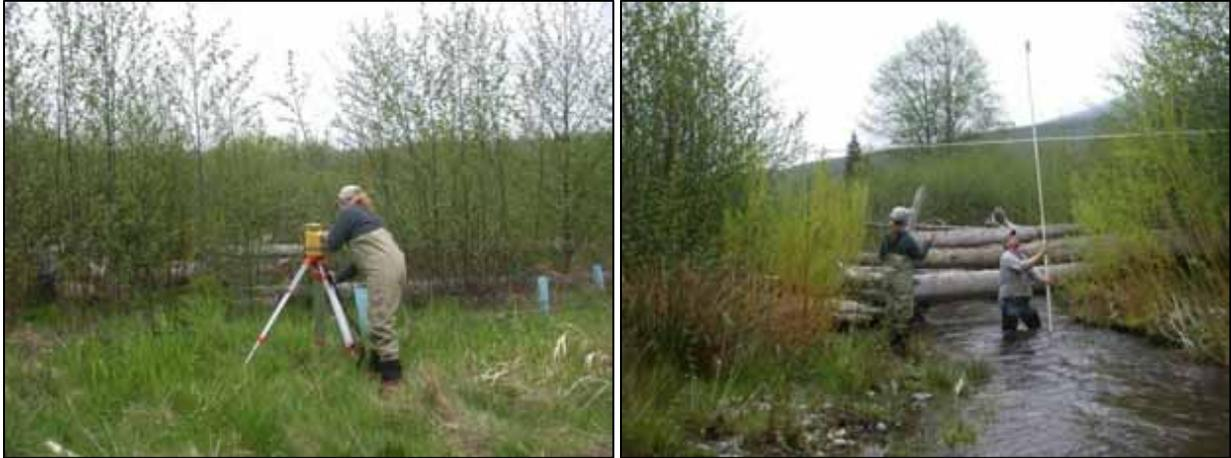
**Figure 2.2. 2008 cross-section survey photos. Left photo: setting up laser level. Right photo: measuring channel bed elevation in JCL Creek (photos by Byron Rot).**
