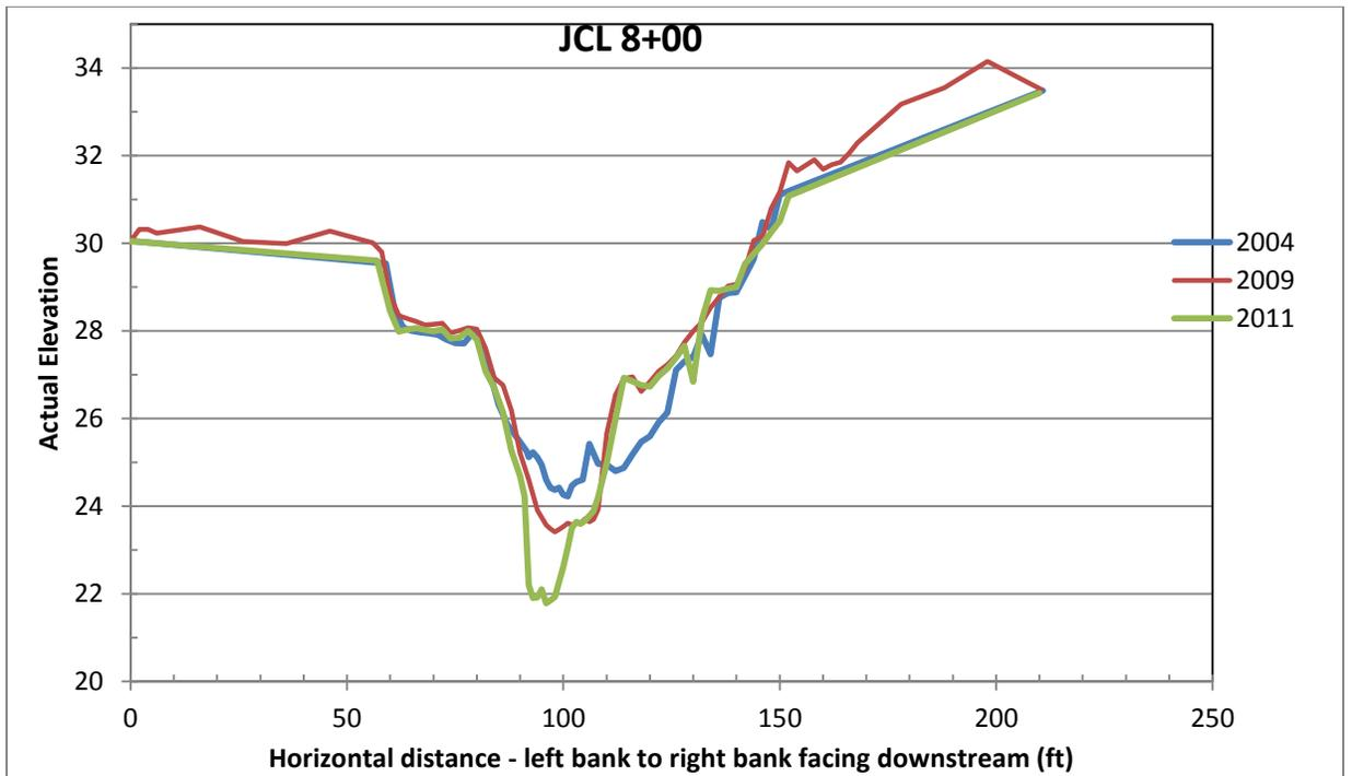
Figure 2.6. Sample JCL channel cross-section (JCL 8+00) for the years 2004, 2009 and 2011.
