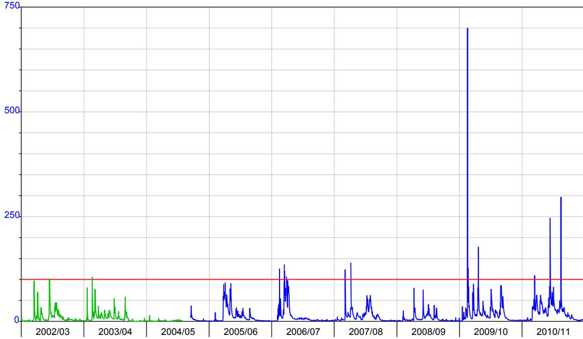
**Figure 1.2. JCL hydrograph for the period of record, years 2002-2011. The DOE gage for October 2002 – April 2005 was in the old JCL channel about 150 ft downstream of Hwy 101. From June 2005 – September 2011 the DOE gage was in the new JCL channel about 500 ft upstream of Hwy 101.**
