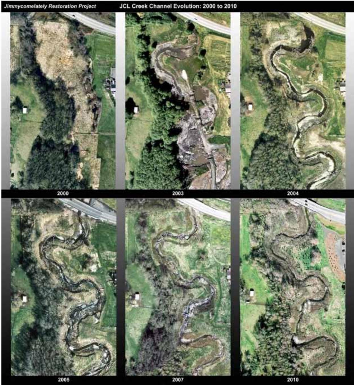
Figure 2. 11. JCL channel evolution from 12+00 to Hwy 101. Photos are pre-project – 2000, during construction – 2003, spring 2004 prior to channel opening in the fall, spring 2005 following channel opening in October 2004, spring 2007, and spring 2010 (graphic by Randy Johnson).
