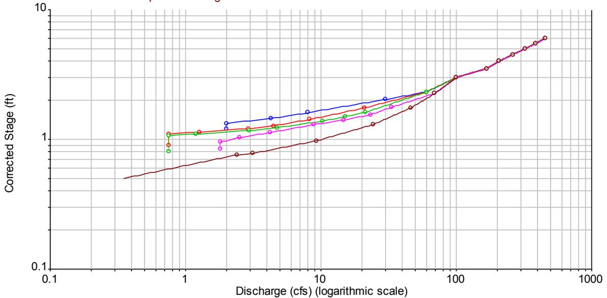
**Figure 1.4. Rating plot on a log-log scale for WY 2009 and 2010. These curves change with channel erosion and deposition. The curve establishes the relationship of stage height to discharge at the DOE stream gage.**
