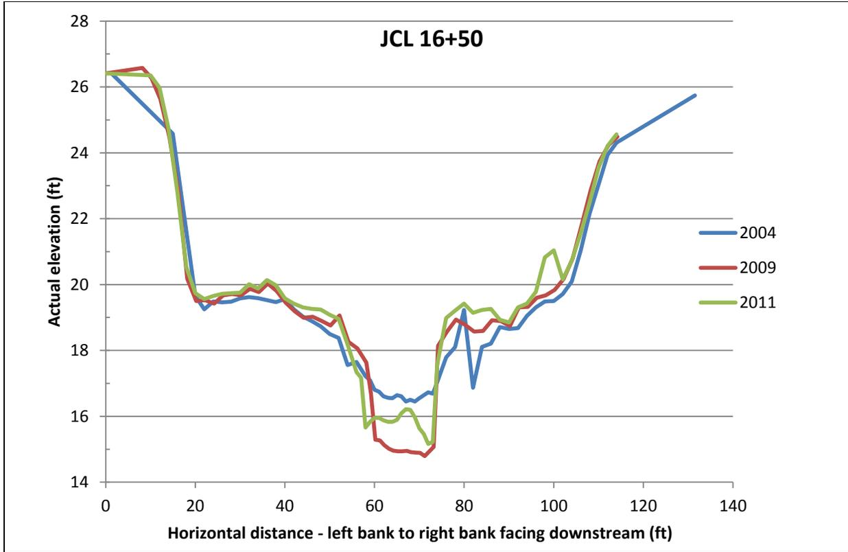
Figure 2.7. Sample JCL channel cross-section (JCL 16 + 50) for the years 2004, 2009 and 2011.
