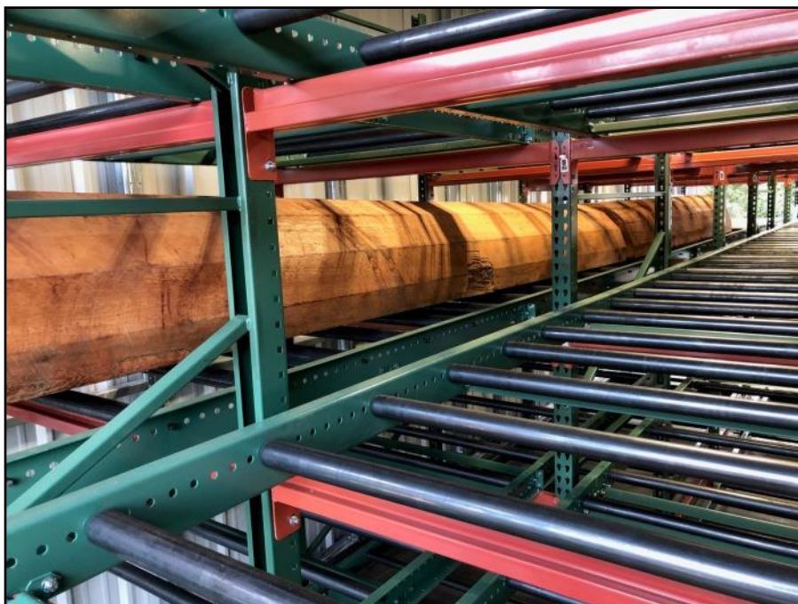
Below, the roller racks with a huge cedar log being pushed in by a forklift.
