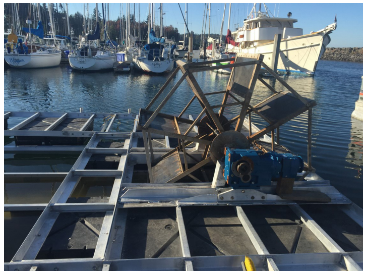
Above, the upwelling action of the FLUPSY is produced by this paddle wheel.
