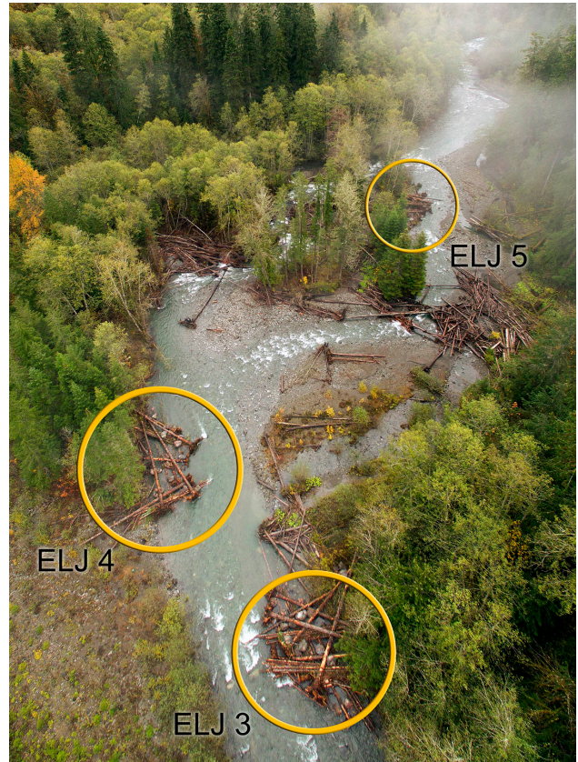
Left, Jamestown Excavating builds the rock-collar anchoring system. Right, engineered log jams on the Dungeness River are circled in yellow.
