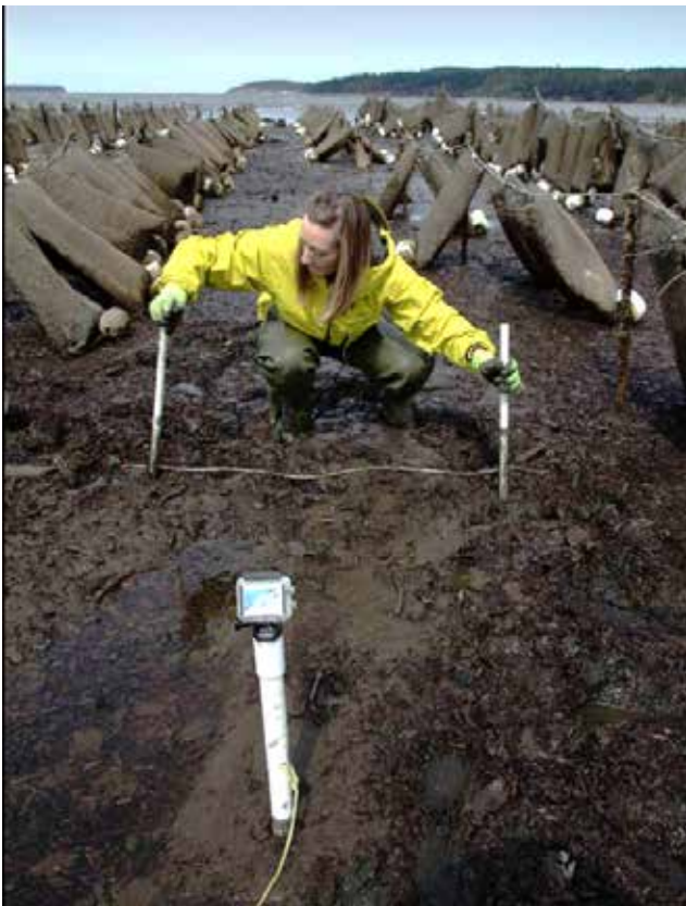
Underwater GoPro video cameras being installed at low tide
