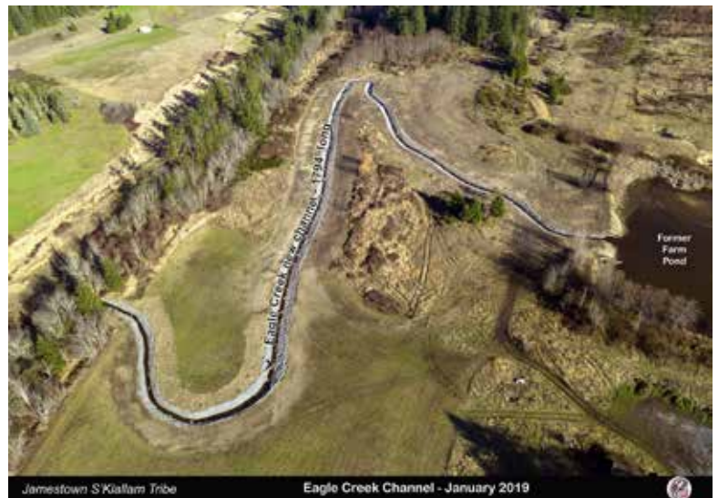
The new open channel constructed at Eagle Creek is 1,794 feet long. It replaces an undersized, below-ground pipe that was approximately 700 feet long. This graphic shows the new channel viewed from the west. Highway 101 is not shown in the image, but is to the right of the pond.
