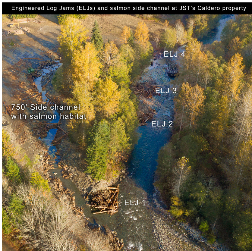
Caldero - At River Mile 9.5 of the Dungeness River, a side channel was recreated to provide improved habitat, especially for juveniles. Several logjams were installed and legacy riprap from earlier shoreline armoring was removed.
